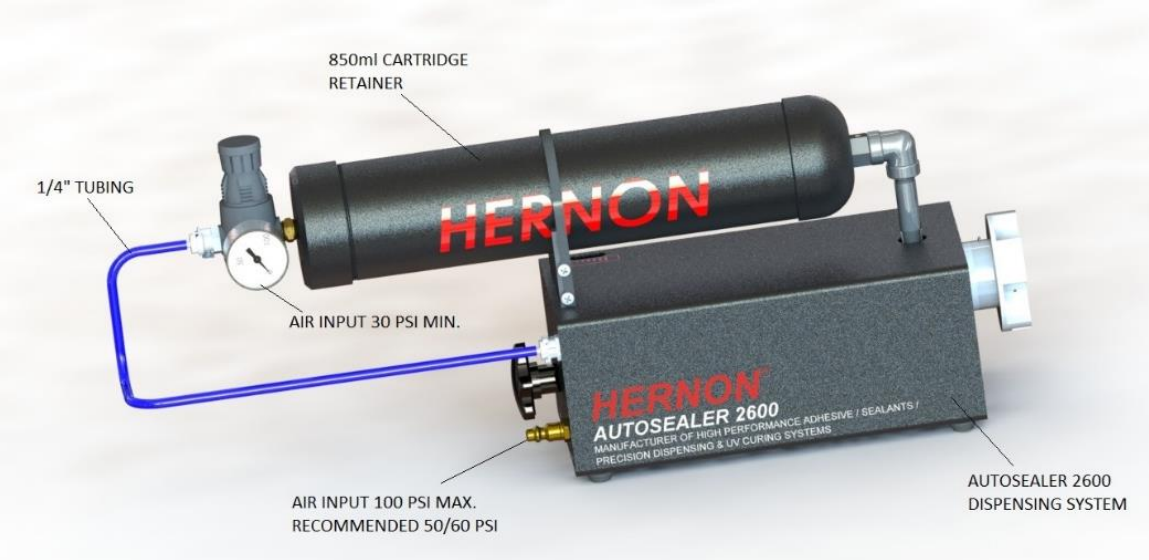
Figure 1- Autosealer 2600, with components labeled.
